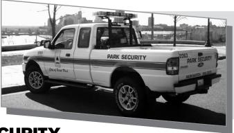
Two new Park Security vehicles were added to the fleet in 2007. These new vehicles are part of a scheduled replacement program through the City fleet services and are replaced every 3 - 4 years. The vehicles are equipped with special light bars for security functions and directional arrows for traffic control, have parks radios mounted inside and list the ParkWatch number on the rear tailgate.
